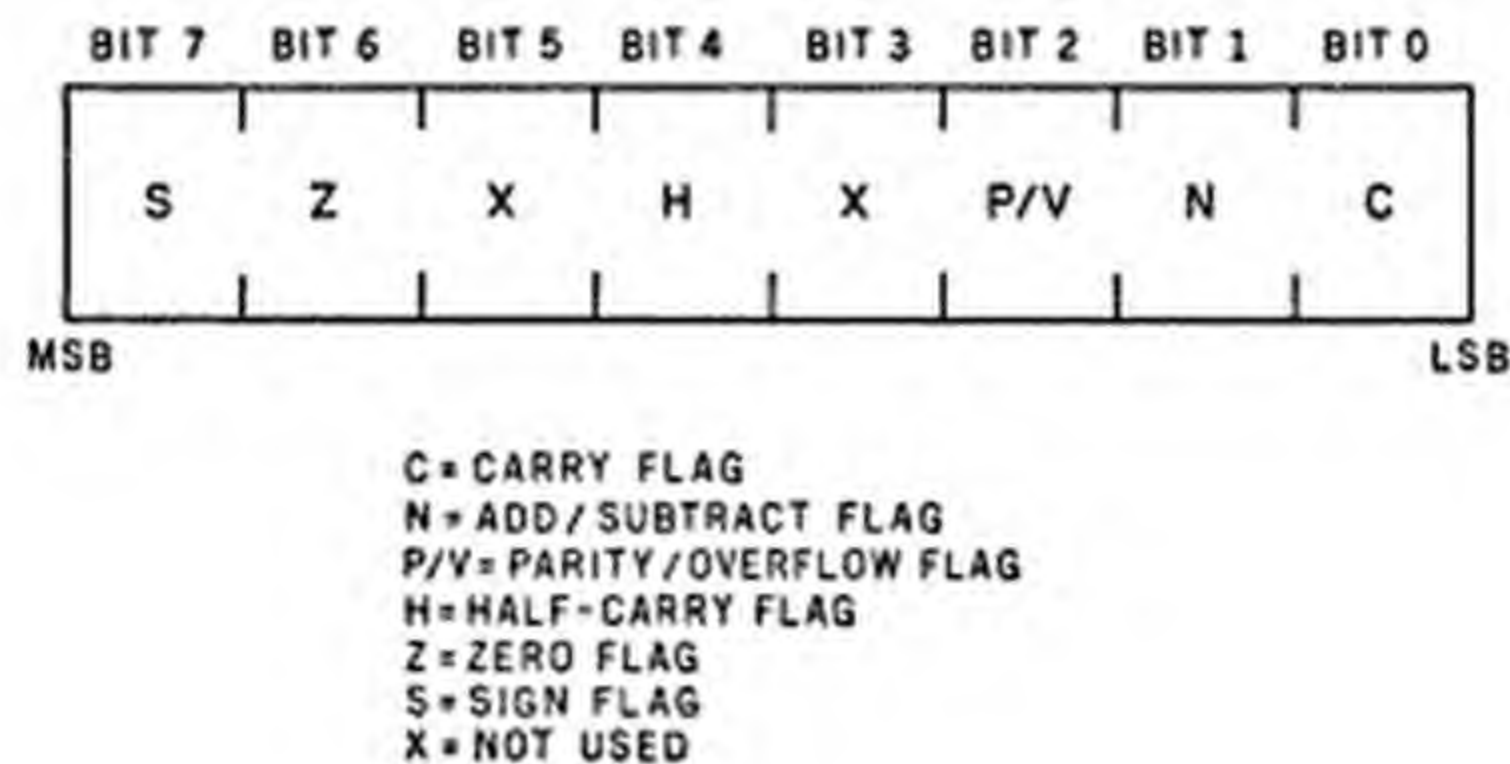
Figure 3.6 Position and identity of status flag bits in the flag register.
